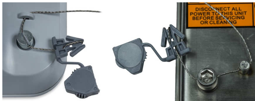
Figure A-42: Seal Installation, IND231 (left) and IND236 (right)
