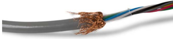
Figure A-26: Load Cell Cable with Shield Wire Folded Back
