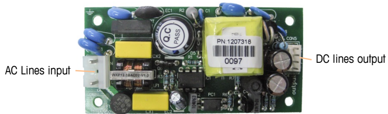
Figure A-17: Power Board
