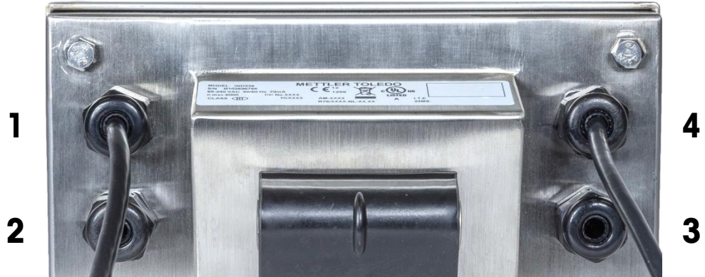
Figure A-14: IND236 Enclosure Openings
