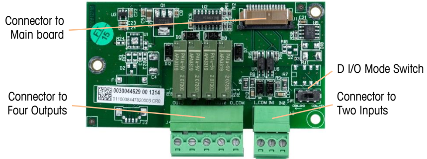
Figure A-36: Discrete I/O Option Board
